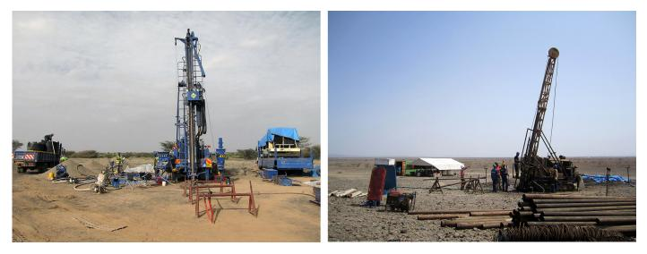
Figure 7. Photos of the HSPDP drilling operations. Left: West Turkana (WTK) site using a truck-mounted PRD Multistar drilling rig operated by Drilling and Prospecting International (DPI) used for all Kenyan drilling campaigns (photo credit: Craig Feibel). Right. Northern Awash (NAO) site using a track mounted Christensen CS14 drilling rig operated by Geosearch (now Orezone Drilling) used for Ethiopian campaigns (photo credit: Beau Marshall).
