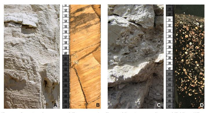
**Figure 10.** Comparison of outcrop versus drill core preservation. Close-up of diatomite outcrop adjacent to drilled Tugen Hills sequence (A) and laminated diatomite from BTB13-1A (B). Close-up of coquina adjacent to drilled West Turkana sequence (C) and coquina from WTK13-1A (D). Note that outcrop examples may not reflect exact correlates of drill core examples.
